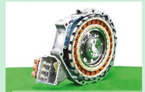
Alicyclic epoxy for EV motors (application example)
